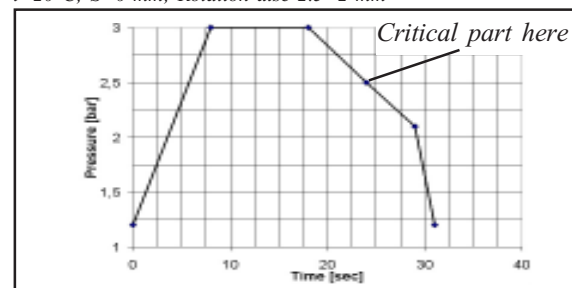
Fig. 3: An example of a pressure cycle to be repeated continuously.
