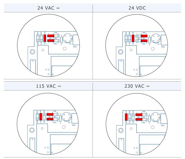
The output voltages 115Vac or 230Vac is not available in 24VAC or 24VDC power input models,
