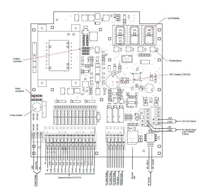
Note: If the Control Unit is a +24Vdc power-supplied model, please connect:
